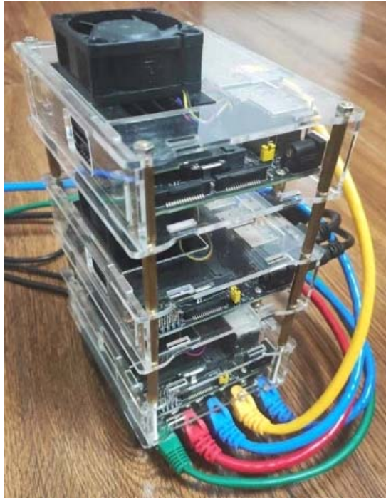
Fig. 5. Design of architecture of the distributed computational NVIDIA Jetson based GPU-accelerated clustering system
